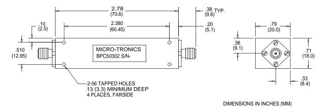
Micro-Tronics Model BPC50302 was specifically designed to pass 3600 to 4200 MHz while maintaining low insertion loss and sharp rejection. The basic bandpass filter design can also be adapted to custom applications.
