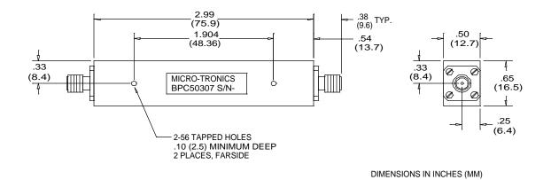
Micro-Tronics Model BPC50307 was specifically designed to pass 12250 to 12750 MHz while maintaining low insertion loss and sharp rejection. The basic bandpass filter design can also be adapted to custom applications.
