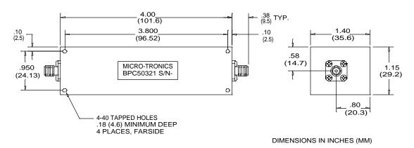
Micro-Tronics Model BPC50321 was specifically designed to pass 1435 to 1540 MHz while maintaining low insertion loss and sharp rejection. The basic bandpass filter design can also be adapted to custom applications.
