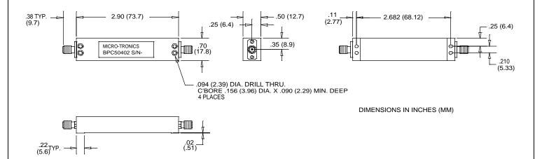
Micro-Tronics Model BPC50402 was specifically designed to pass 2.00 to 6.00 GHz while maintaining low insertion loss and sharp rejection. The basic bandpass filter design can also be adapted to custom applications.
