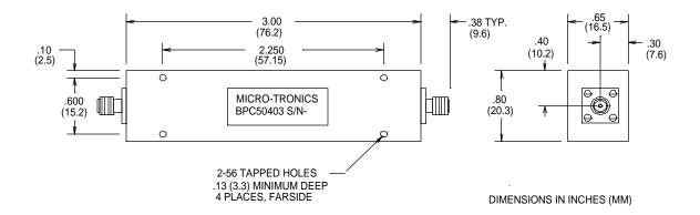
Micro-Tronics Model BPC50403 was specifically designed to pass 4.00 to 8.00GHz while maintaining low insertion loss and sharp rejection. The basic bandpass filter design can also be adapted to custom applications.
