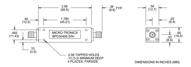
Micro-Tronics Model BPC50406 was specifically designed to pass 8.00 to 12.00 GHz while maintaining low insertion loss and sharp rejection. The basic bandpass filter design can also be adapted to custom applications.
