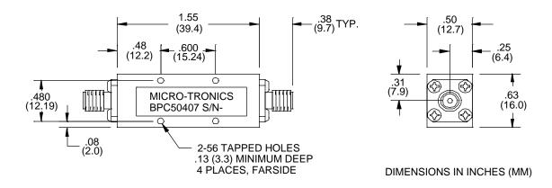
Micro-Tronics Model BPC50407 was specifically designed to pass 8.00 to 16.00GHz while maintaining low insertion loss and sharp rejection. The basic bandpass filter design can also be adapted to custom applications.
