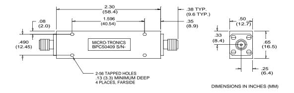
Micro-Tronics Model BPC50409 was specifically designed to pass 10.0 to 14.0 GHz while maintaining low insertion loss and sharp rejection. The basic bandpass filter design can also be adapted to custom applications.
