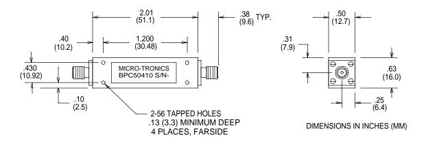
Micro-Tronics Model BPC50410 was specifically designed to pass 10.00 to 15.00 GHz while maintaining low insertion loss and sharp rejection. The basic bandpass filter design can also be adapted to custom applications.
