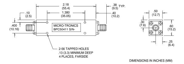
Micro-Tronics Model BPC50411 was specifically designed to pass 12.0 to 18.0GHz while maintaining low insertion loss and sharp rejection. The basic bandpass filter design can also be adapted to custom applications.
