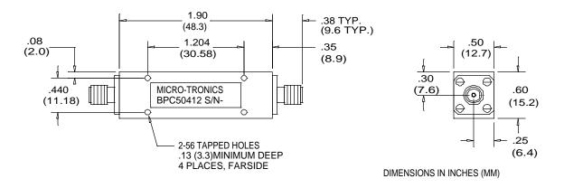
Micro-Tronics Model BPC50412 was specifically designed to pass 14.00 to 18.00 GHz while maintaining low insertion loss and sharp rejection. The basic bandpass filter design can also be adapted to custom applications.
