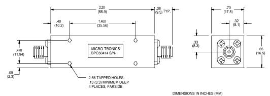
Micro-Tronics Model BPC50414 was specifically designed to pass 4000 to 5000 MHz while maintaining low insertion loss and sharp rejection. The basic bandpass filter design can also be adapted to custom applications.
