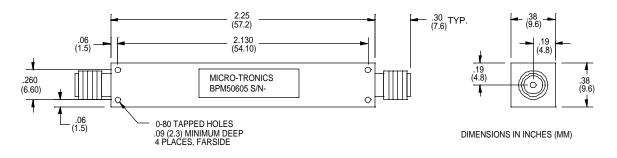
Micro-Tronics Model BPM50605 was specifically designed to pass 950 to 1700 MHz while maintaining low insertion loss and sharp rejection. The basic bandpass filter design can also be adapted to custom applications.
