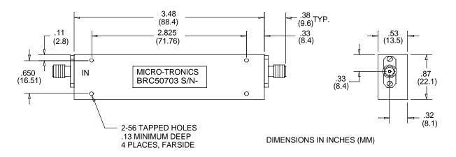
Micro-Tronics Model BRC50703 was specifically designed to reject the 5150 to 5350 MHz portion of the IEEE 802.11A band while maintaining low insertion loss and a broad upper passband. The basic notch filter design can also be adapted to custom applications the 5000 to 6000 MHz frequency range for similar bandwidths.
