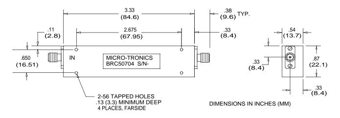
Micro-Tronics Model BRC50704 was specifically designed to reject the 5470 to 5725 MHz portion of the IEEE 802.11A band while maintaining low insertion loss and a broad upper passband. The basic notch filter design can also be adapted to custom applications the 5000 to 6000 MHz frequency range for similar bandwidths.
