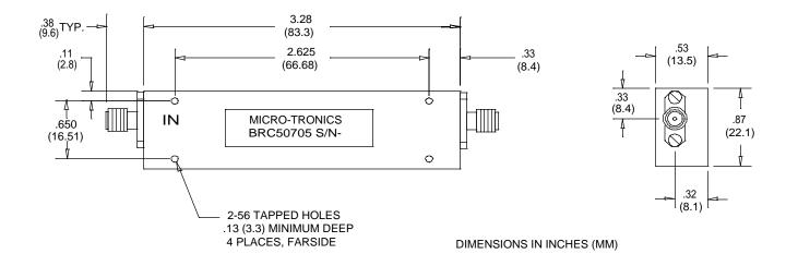
Micro-Tronics Model BRC50705 was specifically designed to reject the 5725 to 5875 MHz portion of the IEEE 802.11A band while maintaining low insertion loss and a broad upper passband. The basic notch filter design can also be adapted to custom applications the 5000 to 6000 MHz frequency range for similar bandwidths.
