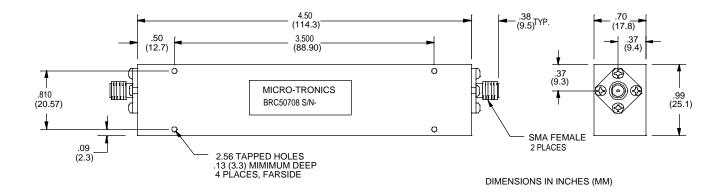
Micro-Tronics Model BRC50708 was specifically designed to reject the 3400 to 3600 MHz portion of the European WIMAX band while maintaining low insertion loss and a broad upper passband. The basic notch filter design can also be adapted to custom applications in the 3000 to 4000 MHz frequency range for similar bandwidths.
