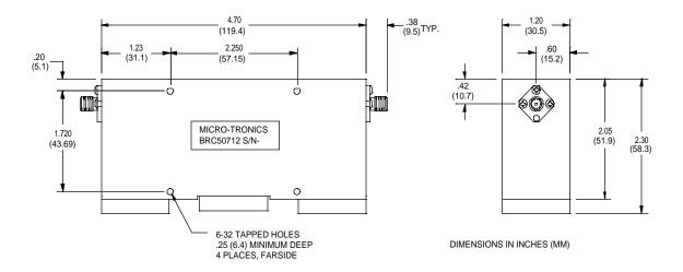
Micro-Tronics Model BRC50712 was specifically designed to reject the GPS L1 band while maintaining low insertion loss and a broad upper passband. The basic notch filter design can also be adapted to custom applications.
