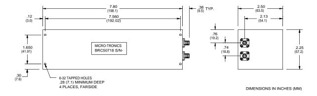
Micro-Tronics Model BRC50718 was specifically designed to reject 880 to 915 MHz (GSM 900, E-GSM) while maintaining low insertion loss and broad upper passband. The basic notch filter design can also be adapted to custom applications.
