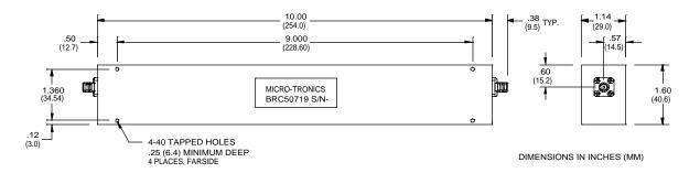
Micro-Tronics Model BRC50719 was specifically designed to reject 1710 to 1785 MHz while maintaining low insertion loss and broad upper passband. The basic notch filter design can also be adapted to custom applications.
