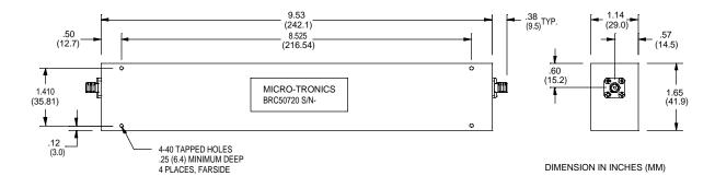
Micro-Tronics Model BRC50720 was specifically designed to reject 1850 to 1910 MHz (PCS 1900) while maintaining low insertion loss and broad upper passband. The basic notch filter design can also be adapted to custom applications.
