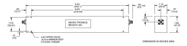
Micro-Tronics Model BRC50721 was specifically designed to reject 1920 to 1980 MHz (UMTS band 1, IMT) while maintaining low insertion loss and broad upper passband. The basic notch filter design can also be adapted to custom applications.
