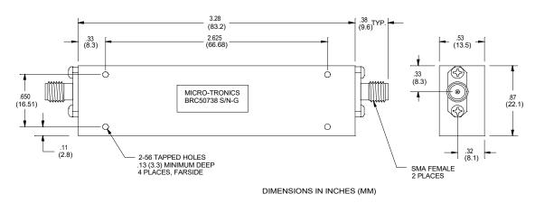
Micro-Tronics Model BRC50738 was specifically designed to reject 5150 to 5250 MHz while maintaining low insertion loss and a broad upper passband. The basic notch filter design can also be adapted to custom applications in the 5000 to 6000 MHz frequency range for similar bandwidths.
