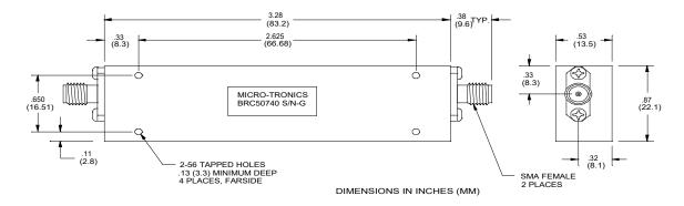
Micro-Tronics Model BRC50740 was specifically designed to reject 5725 to 5850 MHz while maintaining low insertion loss and a broad upper passband. The basic notch filter design can also be adapted to custom applications in the 5000 to 6000 MHz frequency range for similar bandwidths.
