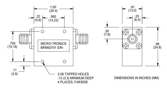
Micro-Tronics Model BRM50701 was specifically designed to reject 2400 to 2500 MHz Bluetooth frequencies while maintaining low insertion loss and broad upper passband. The basic notch filter design can also be adapted to custom applications.
