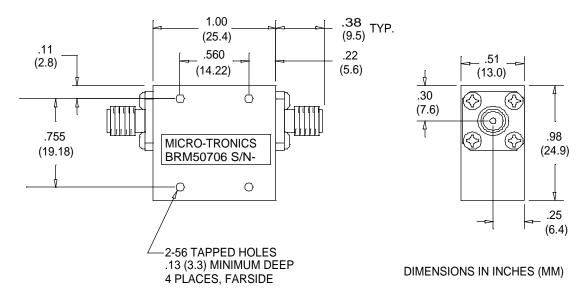
Micro-Tronics Model BRM50706 was specifically designed to reject 800 to 1000 MHz while maintaining low insertion loss and broad upper passband. The basic notch filter design can also be adapted to custom applications.
