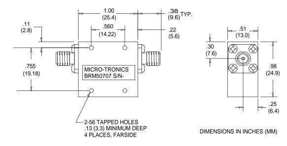
Micro-Tronics Model BRM50707 was specifically designed to reject 1800 to 2000 MHz while maintaining low insertion loss and broad upper passband. The basic notch filter design can also be adapted to custom applications.
