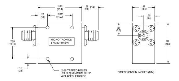
Micro-Tronics Model BRM50710 was specifically designed to reject the 2300 to 2400 MHz portion of the IEEE 802-16 band while maintaining low insertion loss and broad upper passband. The basic notch filter design can also be adapted to custom applications.
