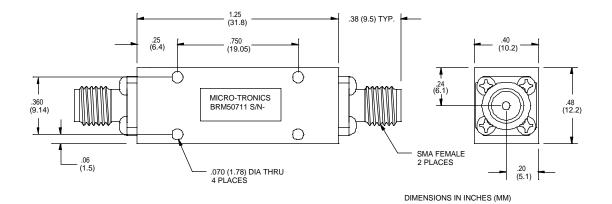
Micro-Tronics Model BRM50711 was specifically designed to reject the 3400 to 3800 MHz portion of the IEEE 802-16 band while maintaining low insertion loss and broad upper passband. The basic notch filter design can also be adapted to custom applications.
