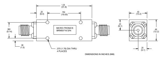
Micro-Tronics Model BRM50716 was specifically designed to reject 5150 to 5880 MHz while maintaining low insertion loss and broad upper passband. The basic notch filter design can also be adapted to custom applications.
