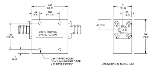
Micro-Tronics Model BRM50723 was specifically designed to reject 2110 to 2170 MHz while maintaining low insertion loss and broad upper passband. The basic notch filter design can also be adapted to custom applications.
