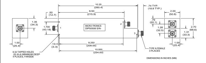
Micro-Tronics Model DIP50508 was specifically designed to pass 1750-1850 MHz and 2200-2300 MHz while maintaining low insertion loss and sharp rejection. The basic Diplexer design can also be adapted to custom applications.
