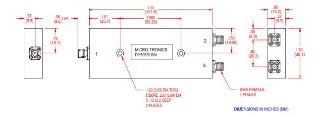
Micro-Tronics Model DIP50520 was specifically designed to pass 4.4-4.625 GHz and 4.475-5.0 GHz while maintaining low insertion loss and sharp rejection. The basic Data Link Diplexer design can also be adapted to custom applications.
