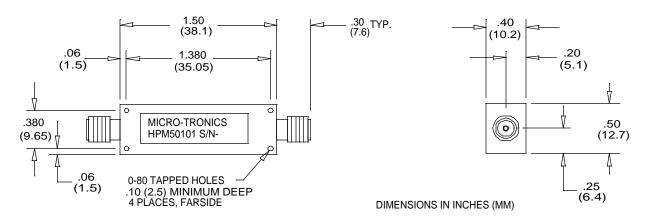
Micro-Tronics Model HPM50101 was specifically designed to reject DC to 80 MHz while maintaining low insertion loss and a broad upper passband. The basic highpass filter design can also be adapted to custom applications.
