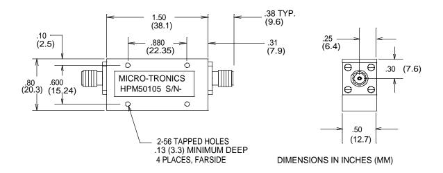
Micro-Tronics Model HPM50105 was specifically designed to reject DC to 6 GHz while maintaining low insertion loss and a broad upper passband. The basic highpass filter design can also be adapted to custom applications.
