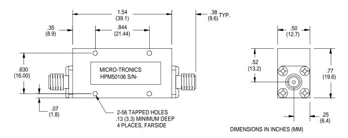
Micro-Tronics Model HPM50106 was specifically designed to reject DC to 5.85 GHz and pass 7 GHz while maintaining low insertion loss and a broad upper passband. The basic highpass filter design can also be adapted to custom applications.
