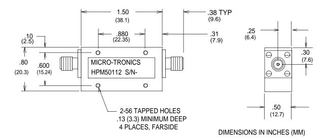
Micro-Tronics Model HPM50112 was specifically designed to reject DC to 5850 MHz while maintaining low insertion loss and a broad upper passband. The basic highpass filter design can also be adapted to custom applications.
