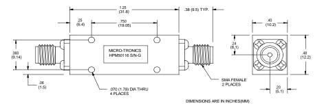
Micro-Tronics Model HPM50116 was specifically designed to reject DC to 2700 MHz while maintaining low insertion loss and a broad upper passband. The basic highpass filter design can also be adapted to custom applications.
