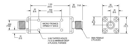
Micro-Tronics Model HPM50117 was specifically designed to reject DC to 2700 MHz while maintaining low insertion loss and a broad upper passband. The basic highpass filter design can also be adapted to custom applications.
