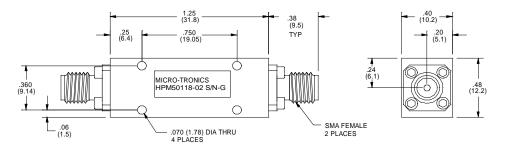
Micro-Tronics Model HPM50118 was specifically designed to reject DC to 3300 MHz while maintaining low insertion loss and a broad upper passband. The basic highpass filter design can also be adapted to custom applications.
