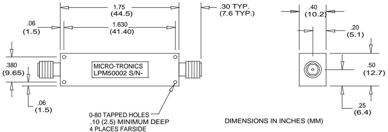
Micro-Tronics Model LPM50002 was specifically designed to pass DC to 230 MHz and reject 310 MHz, while maintaining low insertion loss and a broad upper stopband. The basic lowpass filter design can also be adapted to custom applications.
