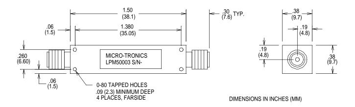
Micro-Tronics Model LPM50003 was specifically designed to pass DC to 425 MHz and reject 500 MHz, while maintaining low insertion loss and a broad upper stopband. The basic lowpass filter design can also be adapted to custom applications.
