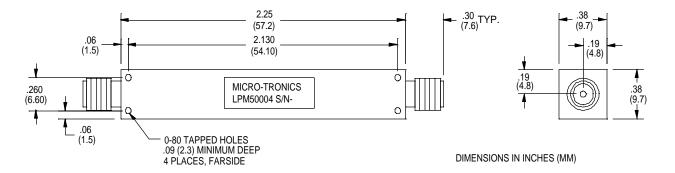
Micro-Tronics Model LPM50004 was specifically designed to pass DC to 1000 MHz and reject 1500 MHz, while maintaining low insertion loss and a broad upper stopband. The basic lowpass filter design can also be adapted to custom applications.
