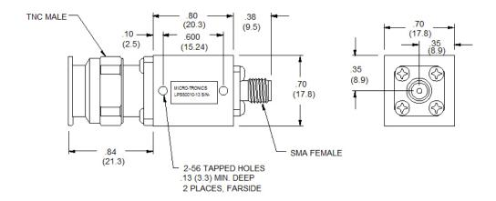
Micro-Tronics Model LPS50010-13 was specifically designed to pass DC to 18 GHz and reject 19.3-20.4 GHz, while maintaining low insertion loss. The basic lowpass filter design can also be adapted to custom applications.
