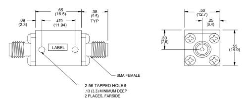
Micro-Tronics Model LPS50010 was specifically designed to pass DC to 18 GHz and reject 19.3-20.4 GHz, while maintaining low insertion loss. The basic lowpass filter design can also be adapted to custom applications.
