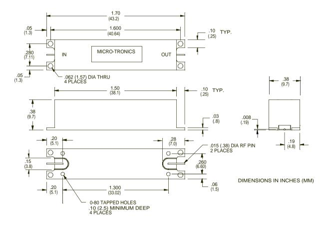
Many of Micro-Tronics lowpass, highpass, and miniature bandpass filters are available in surface mount configuration. The drawing above represents an example of one of our standard surface mount packages. It features a robust machined aluminum case with glass to metal seals to make a sealed unit. It also features solderable ground tabs as well as tapped holes for a variety of mounting options.
